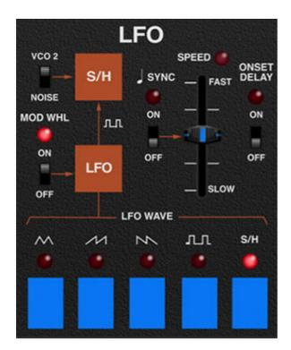
The LFO (low-frequency oscillator) generates sub-audio range signals for modulation purposes. The Quadra contains just one LFO; it can modulate the Poly Synthesizer and/or Lead Synthesizer parameters, depending on current settings.
